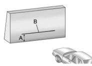
4. At the wall, measure from the ground upward (A) to the recorded distance from Step 3 and mark it.  Draw or tape a horizontal line (B) on the wall the width of the vehicle at the height of the mark in Step 4.
